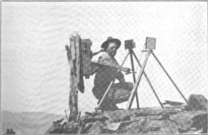
Junction of phone and heliograph systems on national forests. (Photo by courtesy U. S. Forest Service.)
