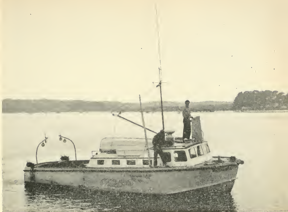
The department's newest research vessel, M. V. Broodbill . The Broodbill is 36 feet long, 15 tons net weight, powered by a Chrysler Crown 106 horsepower engine and has a cruising speed of approximately eight knots. The boat can be controlled from the topside (note wheel in crewman's hand) or from inside the cabin. Salmon gurdies and pulleys are visible at the stern. The Broodbill is used in the abalone, crab and salmon studies.
