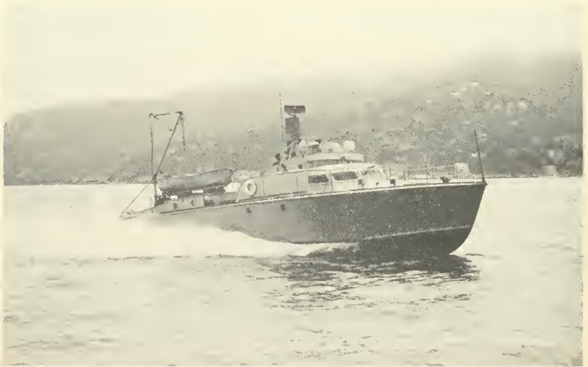
The patrol boat Bonito is newest of the three 63-foot vessels operated by the department in ocean waters. Radar equipment on these boats and on the larger Albacore has been of great value in night patrol work and especially during foggy weather. Photo courtesy of General Electric Company.
