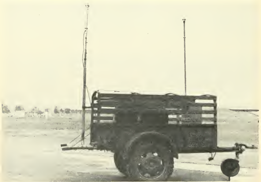
Mobile radio repeater station, with self-contained power plant. This equipment is used in remote areas, where power is not available, to permit continuous transmission and reception.
