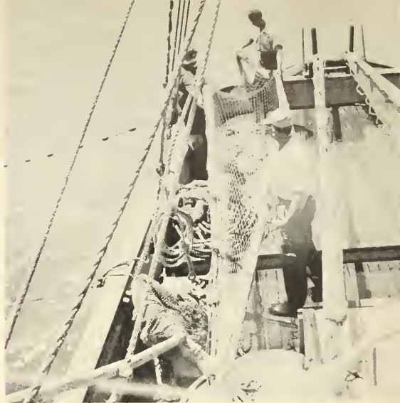
The Porter seine, a new type of net used in daytime airplane fishing, is highly efficient for catching anchovies, sardines and jack mackerel. Wings of the net are being hoisted over the stern with vertical power gurdies.
