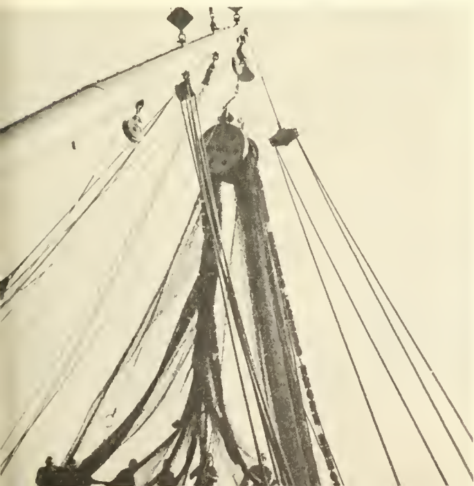
A purse seine net puller, developed and patented during the biennium, enables the fisherman to purse and pull an empty net in as little as 15 minutes, a task that formerly required as much as three hours. (Fish and Game Photo by Anita Daugherty)
