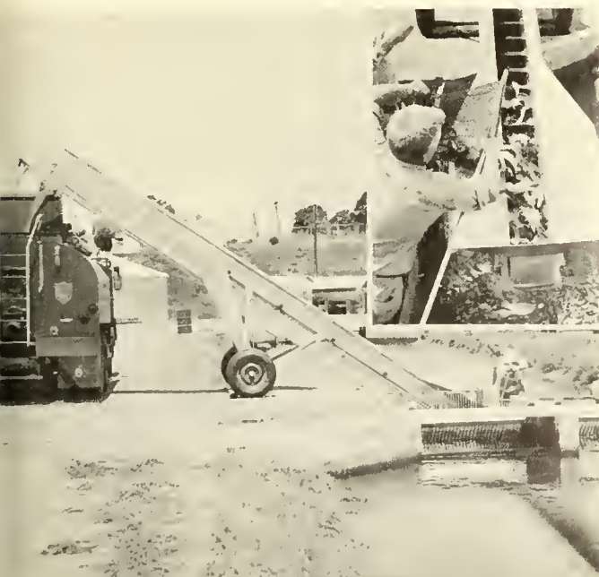
Two time-consuming jobs—loading and weighing of hatchery produced trout for planting—are combined into one by the "escaweigher," which cuts time taken by previous operations by two-thirds. Inset shows cleated rubber conveyor belt.
